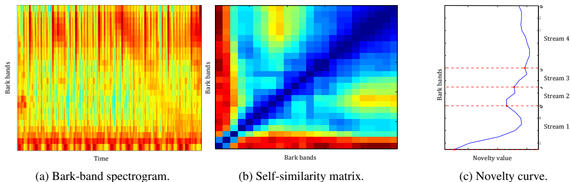
Figure 3: Detection of rhythmic streams using the novelty approach; first a bark-band spectrogram is computed, then its self-similarity matrix, and then the novelty [7] is applied where the novelty peaks define the stream boundaries.
